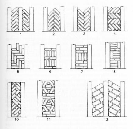
Fig. 17 Common patterns of brick nogging in close studding. (4) Original nogging can be distinguished from restoration work of the nineteenth and twentieth centuries in the same way that the real can always be distinguished from the imitation. Modern bricks are smooth and even, lacking the evidence of exposure to the weather and of piecemeal repair, even if they are of the right size. Both kinds can be seen at Paycocke's (Figs 14 and 15).
