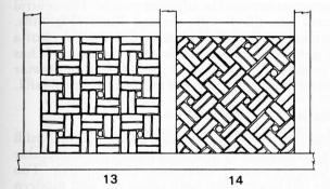
Fig. 18 Hollow squares of paired bricks, upright and oblique, in square framing at nos 28-32, Church Street, Sandwich, Kent. The voids are filled by knapped flints. Now painted.
